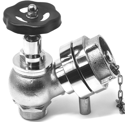
#91.778 Valve 1 1/4" showing with Storz coupling and dust cap N=52 Steel powder coated turning wheel Thread: 1 1/4" BSP. Valve chrome plated brass
