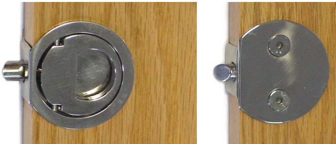
#43.505 Cabinet latch. Flush Slam Latch Mirror Polished 316 Stainless Steel Drill hole: 1 11/16" ~ 43 mm Designed for 3/4 inch ~ 19 mm thick material. All parts high quality 316 stainless steel. Strike plates:
