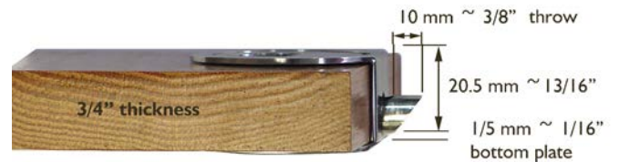
#43.505 Cabinet latch. Flush Slam Latch Mirror Polished 316 Stainless Steel Drill hole: 1 11/16" ~ 43 mm Designed for 3/4 inch ~ 19 mm thick material. All parts high quality 316 stainless steel. Strike plates:
