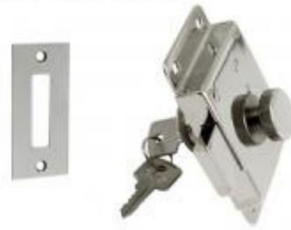
#15.656 Deadbolt rim lock Backset 1 1/2" Cylinder Key/knob For 1" door thickness.
