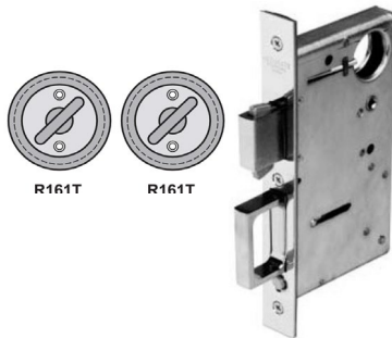
SET: 13.PAR161 Passage set with full mortise mechanism with spring loaded edge pull ; ROUND flush pull with thumb-turns; 2 3/8 inch diameter. MINIMUM DOOR THICKNESS: 1 3/8"
