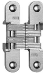
#41.221 Invisible Hinge, minimum door thickness 1 1/8 inch Details: see page 4-1-1-1-C
