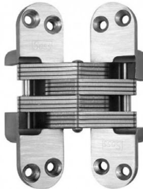
#41.418 Invisible Hinge, minimum door thickness 2 inch. Details: see page 4-1-1-1-A
