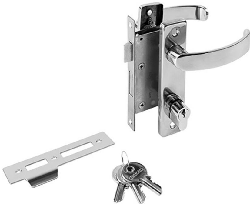
# 11.1615 Marine Grade 316 Stainless Steel Entry Lock with 1 1/2 inch backset (38 mm) with half cylinder and thumb-turn and strike plate
